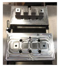
Fig: Mold inserts machined side by side
