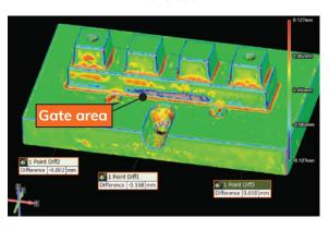
These 3D scans were obtained with Keyence VL series 3D scanner and compared to new inserts after 2500 parts.
