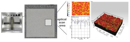
Surface roughness after graphite burning shows a similar finish compared to P20 Steel.
