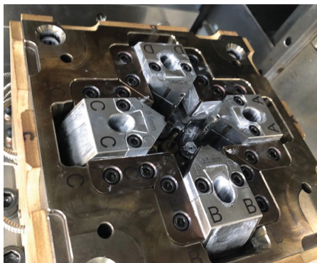
Picture of the assembled mold (left) and molded part (right)
